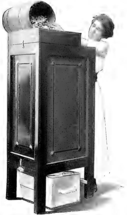
The dust collects in a drawer in the bottom of the hopper and the corks emerge cleaned
